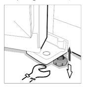
4. Check the alignment of the refrigerator to the surrounding cupboards. The top of the refrigerator should be level from side to side (see diagram below). If you need to adjust the level, use the adjustable rollers as discussed in Step 3.
