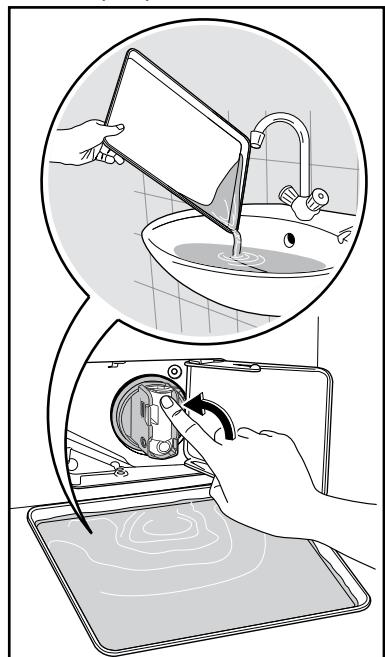
5. Pull back the drainage duct and turn the filter counter-clockwise to remove it.
