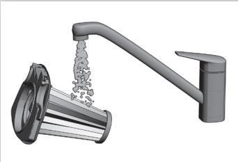
Rinse the filter parts carefully under lukewarm water without using any detergents. (never use the dishwasher or washing machine)
