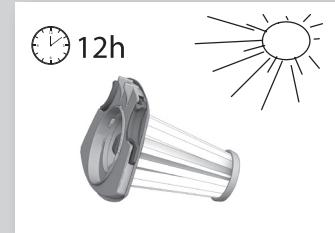
Shake to remove excess water and leave to dry minimum 12h.
