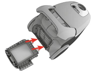
**Note:** Do not use cleaning agents and avoid touching the filter surface Let the filter dry completely (min.12 h In room temperature) before putting back! We recommend to change the the washable filter also at least once in a year or when it is very dirty or damaged.
