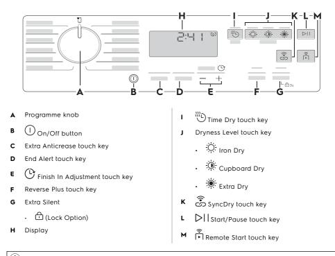
(1) Press the touch buttons with your finger in the area with the symbol or name of the option. Do not wear gloves when you operate the control panel. Make sure that the control panel is always clean and dry.
