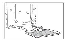
5. When no more water flows, install the inlet hose and the drain hose again.
