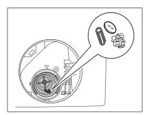
6. Make sure that the impeller of the pump can turn. If this does not occur, contact the service centre.
