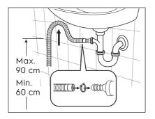
• **Directly into a drain pipe**, at a height of not less than 60 cm and not more than 90 cm.
