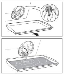
3. When the container is full of water, put the drainage duct back again and empty the container. Do step 2, 3 again and again until no more water flows out from the drain pump.
