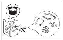
4. Put the front polystyrene packaging element on the floor behind the appliance. Carefully put down the appliance onto its rear side.
