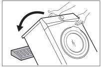
**5.** Remove the polystyrene protection from the bottom.
