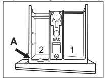
To use also liquid detergent/additive or bleach: Remove detergent divider from the position A and insert it in position B.
