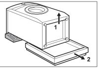
Put the appliance back into an upright position. Remove the power supply cable and the drain hose from the hose holder.
