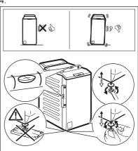
Adjust the appliance correctly to prevent vibration, noise and movement of the appliance when it operates.
