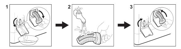
Clean the filter regularly and, especially, if the alarm code  $\vec{E}\vec{e}\vec{u}$  appears on the display.
