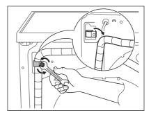
Put the end of the drain and inlet hose in a container. Let the water flow out of the hoses.
