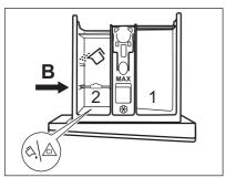
The position **B** of the detergent divider is for powder detergent in the rear compartment and for liquid detergent/additive or bleach in the front compartment.
