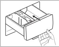
Make sure that the detergent divider is inserted properly and does not cause a blockage when you close the drawer.
