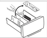
3. Make sure that all detergent residue is removed from the upper and lower part of the recess. Use a small brush to clean the recess.
