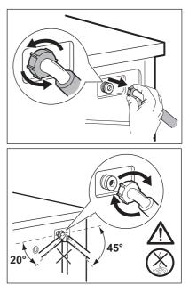
remaining water from the inlet hose and the drain pump.
