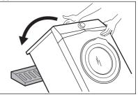
**5.** Remove the polystyrene protection from the bottom.
