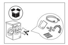
4. Put the front polystyrene packaging element on the floor behind the appliance. Carefully put down the appliance onto its rear side.
