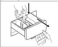
2. Remove the top part of the additive compartment to aid cleaning and flush it out under running warm water, to remove any traces of accumulated detergent. After cleaning, put the top part back into position.
