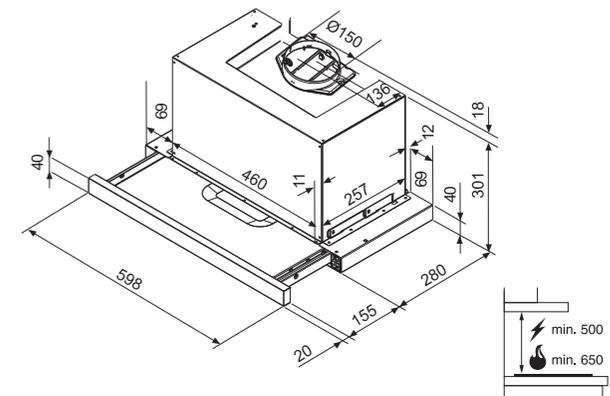
Diameter of exhaust flexible hose cannot be less than 127 mm. 抽風氣喉直徑不可少於127毫米。
