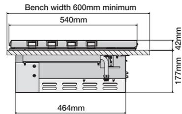
This appliance requires venting. An open area as indicated must be allowed for. A suitable grille can be fitted if desired. This vent area is to allow air into the enclosure for the correct combustion of gases and for the correct exhausting of the products of combustion. The vent must be no less than 700mm x 25mm.
