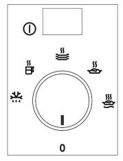
The control panel has a selector and an on/off switch. The control panel is only visible when the drawer is open.
